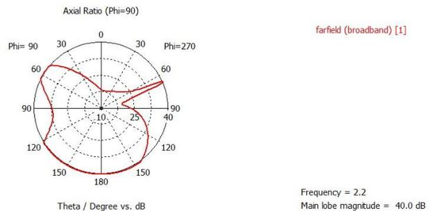
Figure 8: Pattern of Axial Ratio at radiating frequency
