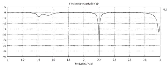
Figure 4: Variation of the magnitude of Return Loss with Frequency
