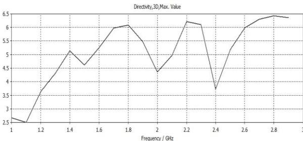
Figure 5: Variation of Directivity (in dB) with Frequency
