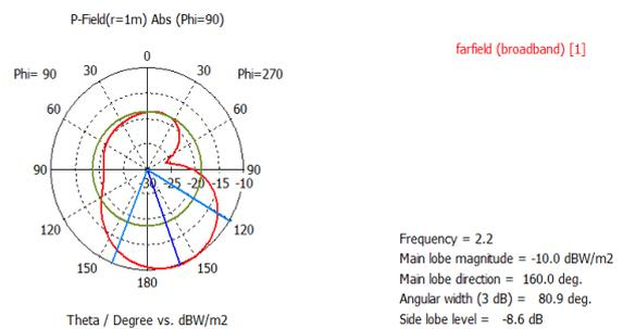
Figure 7: Pattern of Power Density at radiating frequency
