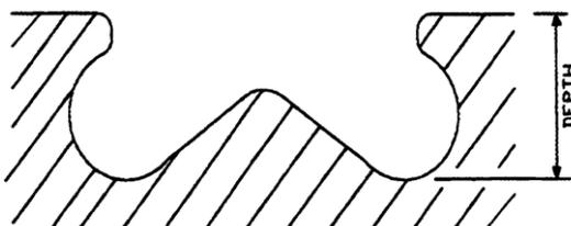
Fig 13: Piston cavity Depth
