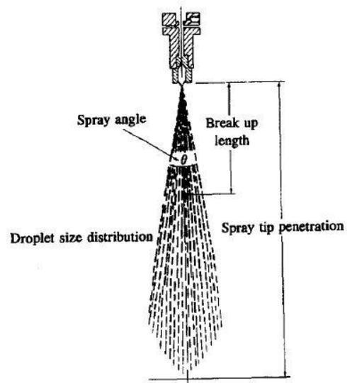
Fig 3: Schematic diagram of fuel spray growth and structure
