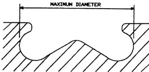
Fig 11: Piston cavity Maximum diameter
