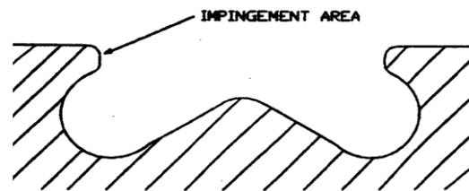
Fig 15: Piston cavity Impingement area
