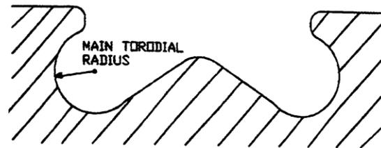
Fig 14: Piston cavity toroidal radius
