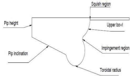
Fig 8: Piston cavity geometrical parameters
