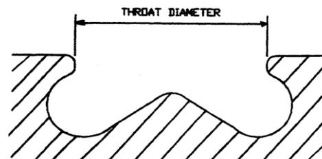
Fig 10: Piston cavity throat diameter
