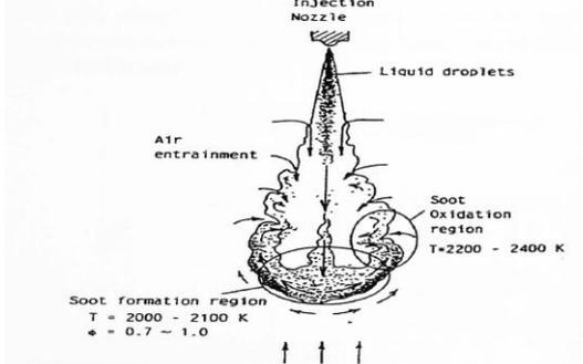
Figure 6: Schematic diagram of soot formation.
