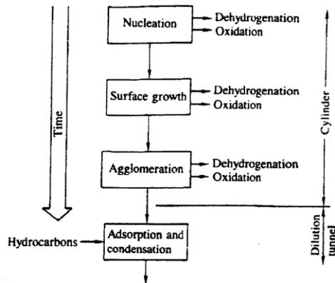
Figure 7: Schematic diagram of particulate formation, from initiation to exhaust-out emission in diesel engines.
