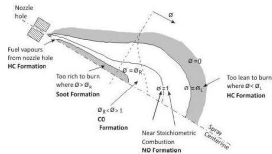
Fig 4: Schematic of a Diesel Injection Spray
