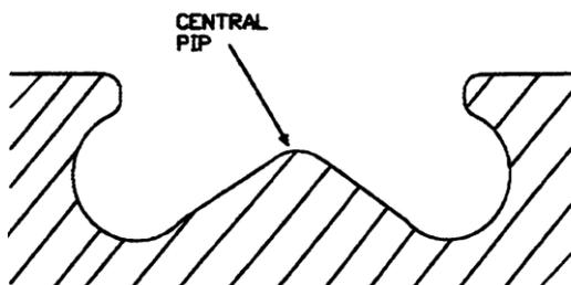
Fig 12: Piston cavity central pip
