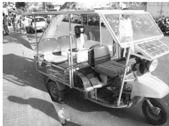
**Fig. 2.** Motor-assisted pedal cycle rickshaw
