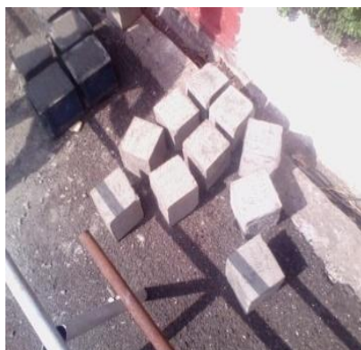
Fig.3 Specimen Sample for Compressive and Flexural Strength.
