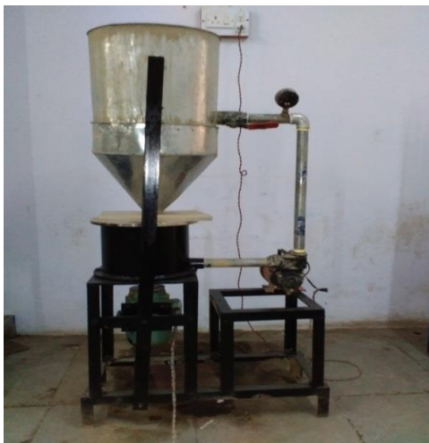
Fig.1 Photograph of jet erosion tester
