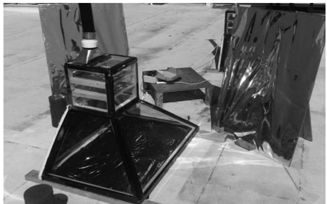
Figure 2. Solar dryer and two concentrating solar reflection panels (James et al 2012)
