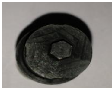
Fig 2.2: Friction stir processing Tool
