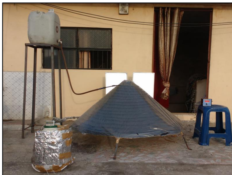
Figure V Actual view of umbrella shape solar hot water device
