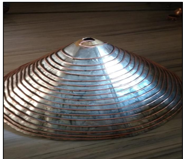
Figure III Actual view of umbrella shape solar collector with spiral tube
