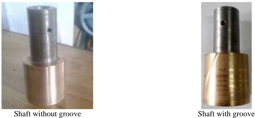
Figure 2 Shaft after Fabrication
