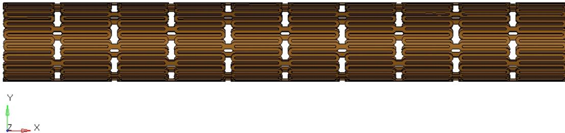
Fig 1 Linear array of 5 instances stent
