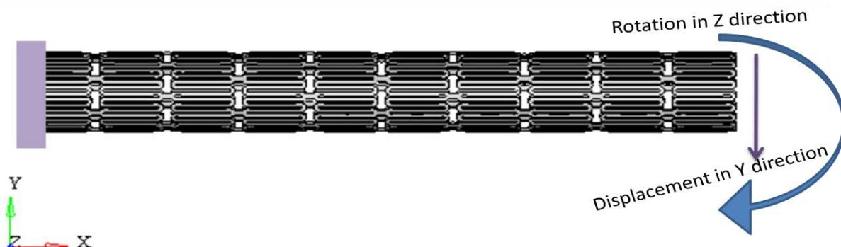
Fig.2 Stent model with loads and boundary conditions
