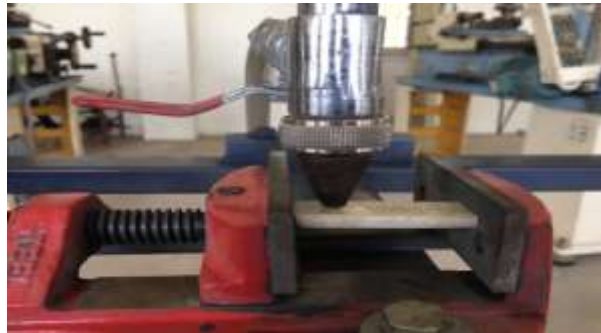
Fig.2.Drill Vice Holding The Workpiece
