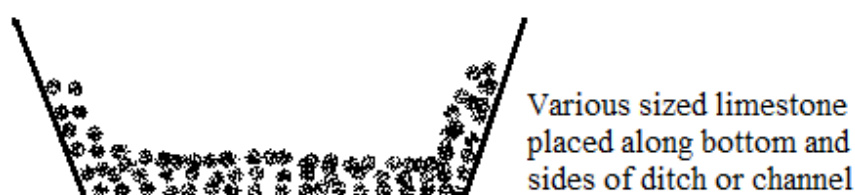
Fig.3. Cross section of an open limestone channel
