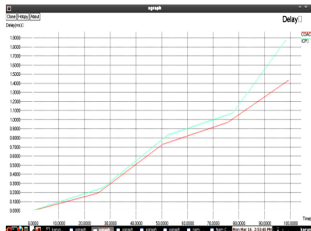
Fig. 11 Time interval between first packet and second packet. It signifies that COACS yields less delay than ICP
