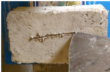
Fig 6: Hardness test for papercrete having 75% of GGBS
