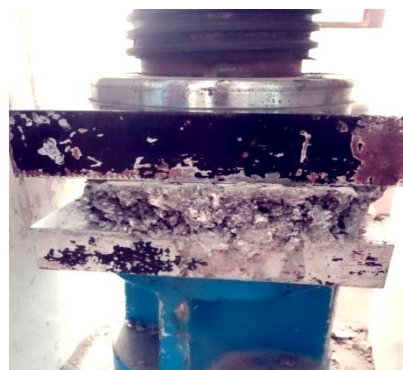
Fig 1: Papercrete brick after a compressive strength test
