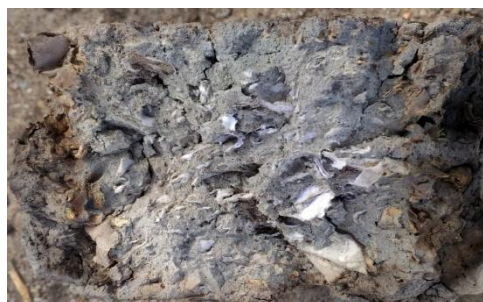
Fig 4: Interior of papercrete after burning
