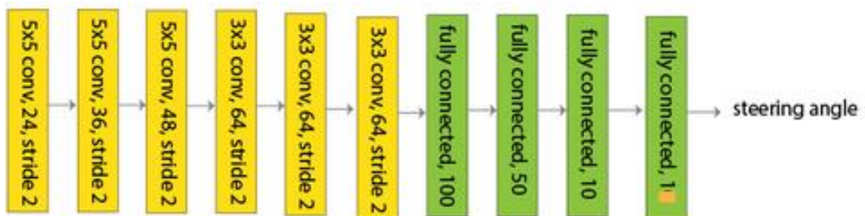
Fig 3: Architecture of CNN model Steering Angle Prediction
