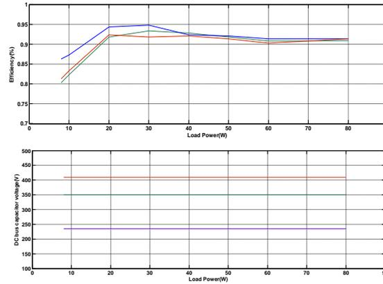
Fig.10 Measured efficiency versus load power for a range of input voltage
