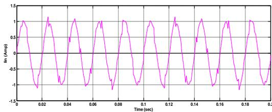
Fig. 8(a) Input current waveform (R Load)
