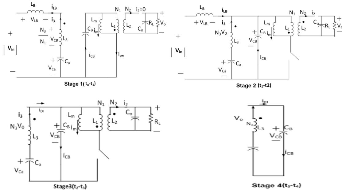
Fig. 4(a) Equivalent circuit operation stages of the proposed PFC circuit during one switching period
