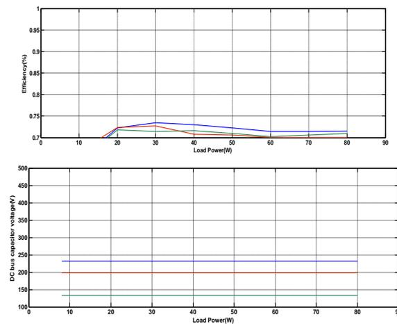
Fig.9 Measured efficiency versus load power for a range of input voltage
