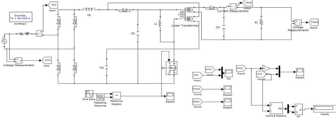
Fig.7 System Model of Proposed converter (R Load) in MATLAB
