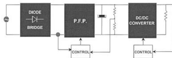
Fig.1 Two stage ac-dc PFC converter.
