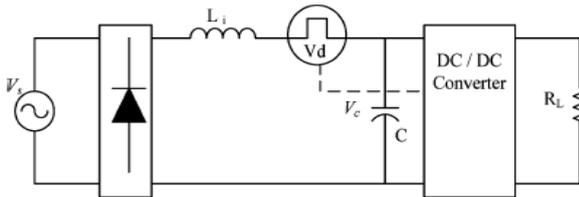
Fig 2 General circuit diagram of diode rectifier with single stage PFC cell.
