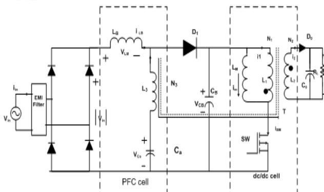
Fig 3 Proposed quasi-active PFC circuit
