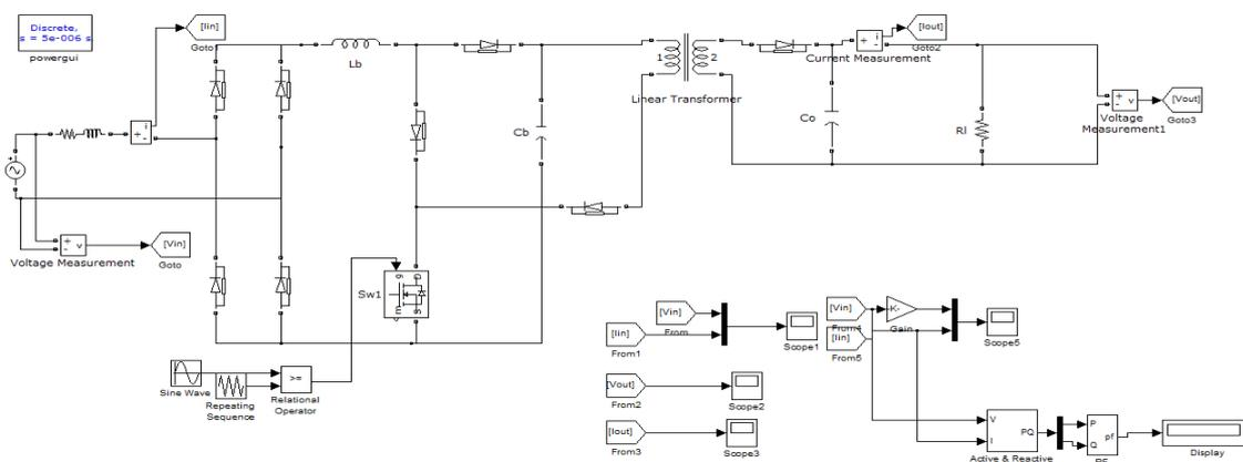
Fig.5 System Model of Boost+flyback converter (R Load) in MATLAB
