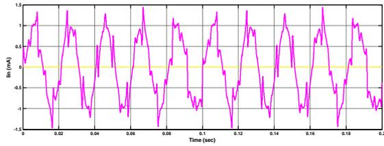
Fig.6 (a) Input current waveform (R Load)
