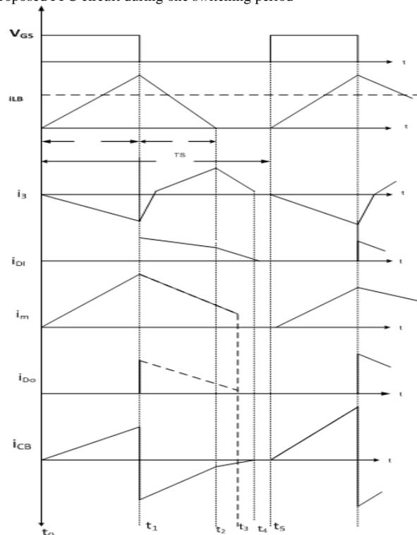
Fig. 4 (b) Key switching waveforms of the proposed PFC technique
