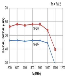
Fig 9: SNDR, SFDR vs Sampling Frequency
