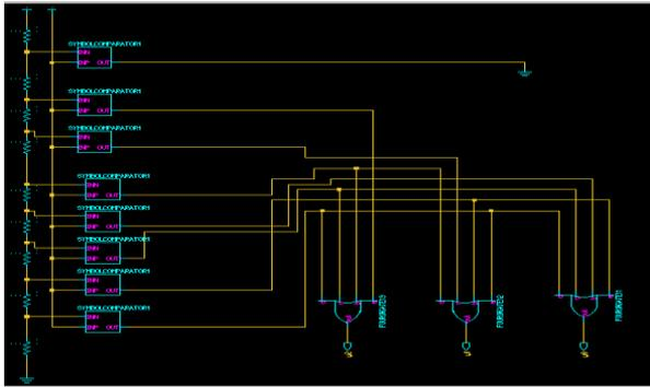
Fig 7: Schematic view of 3bit ADC
