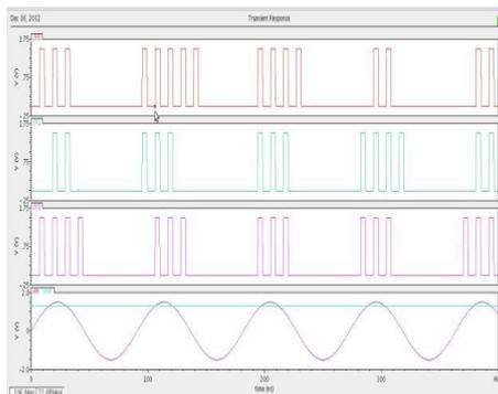
Fig 8: Output Waveform of 3bit ADC
