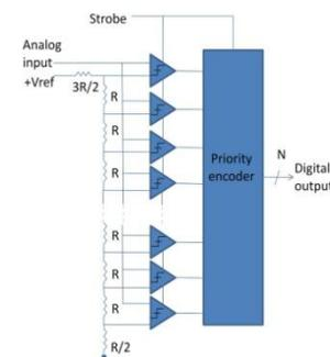
Figure 1: N-Bit Flash ADC
