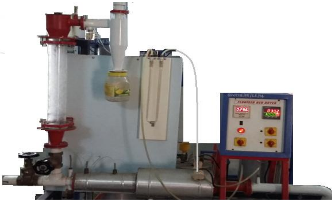
Figure1. Fluidized bed dryer set up for drying conventional material.
