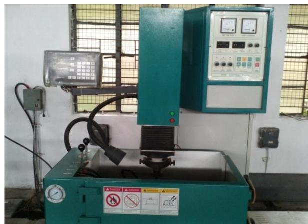
Figure 2: Electric Discharge Machine Setup
