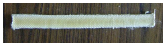
Fig2.5 Vibration analysis test specimen
