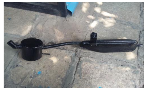
Fig.3.1 Modified Silencer with Turbocharger
