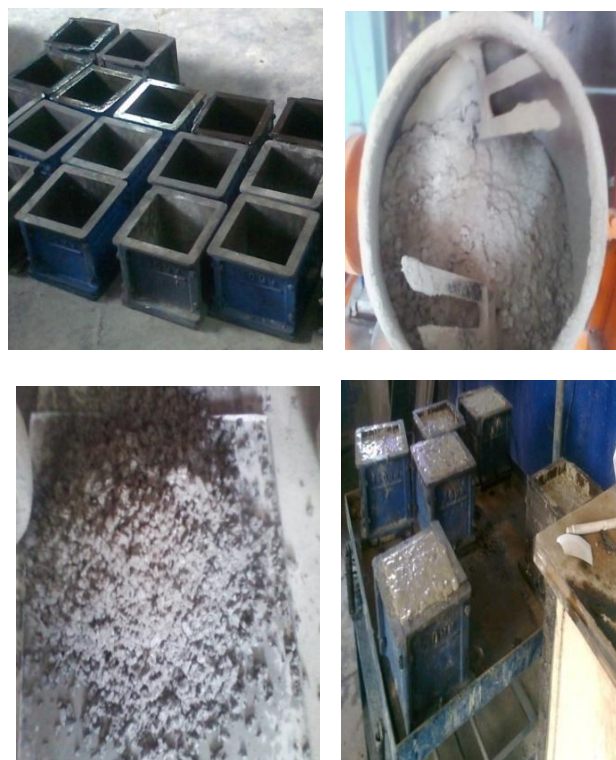
Fig. 2 Making of Sisal Fiber Reinforced Concrete
