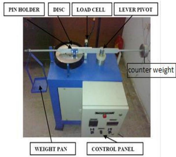
Fig.1. Pin on disc Test-Rig
