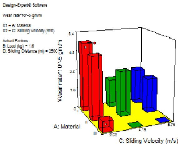
Fig 3: Wear v/s Velocity of sliding
