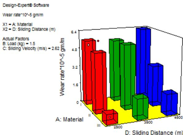
Fig 4: Wear v/s Sliding distance
