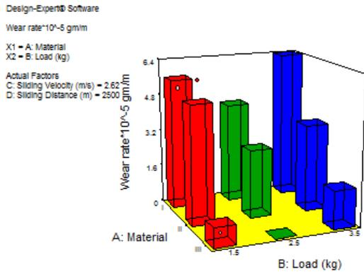
Fig 2: Wear v/s Load
