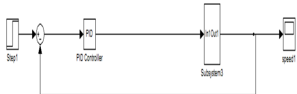
Fig 8 Simulink Model of D.C. Servo Motor using pid controller
