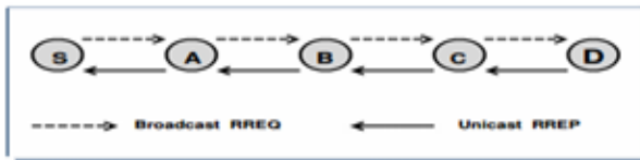
Fig 3: The routing message exchange in AODV
