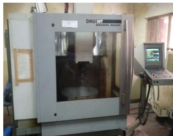
Fig2.3 : Vertical milling machine used for FSW
