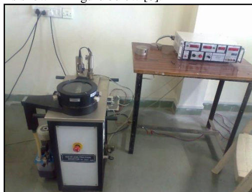
Figure 7: Experimental Setup of Friction and Wear test rig
