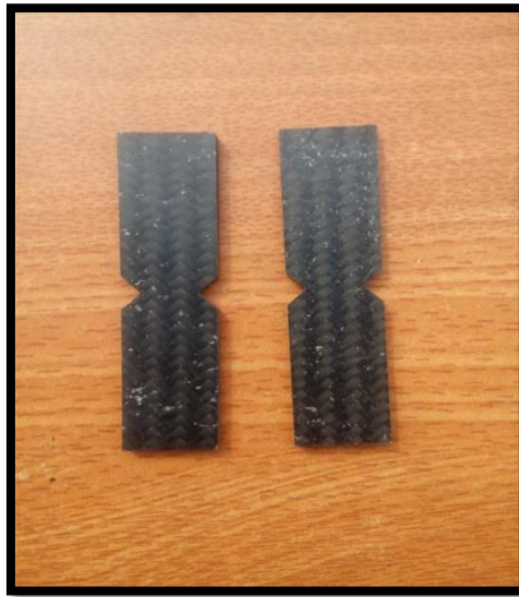
Fig 6: Specimens for shear test
