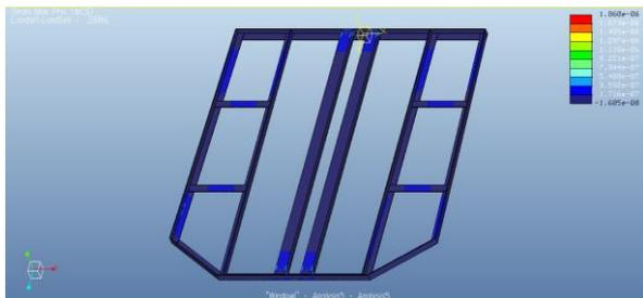
Pic 8: Equivalent elastic strain for magnesium alloy
