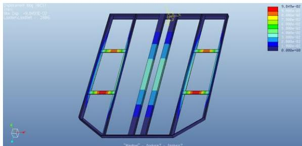
Pic 7: Total deformation for magnesium alloy
