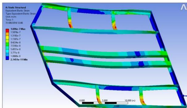
Pic 2: Equivalent elastic strain for the steel chassis
