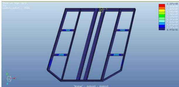
Pic 6: Von-Mises stress for aluminium alloy
