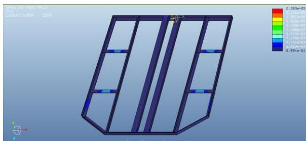
Pic 9: Von-Mises Stress for magnesium alloy
