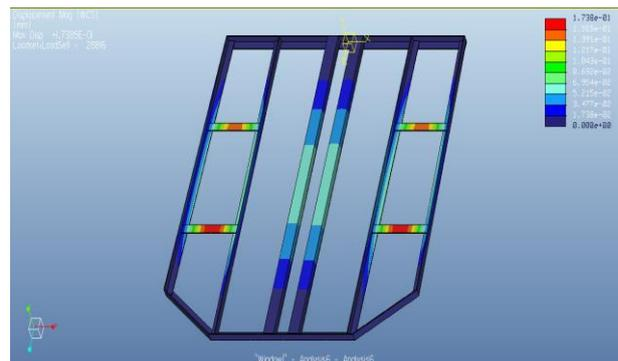
Pic 4: Total deformation for aluminium alloy chassis
