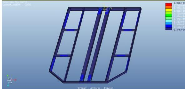
Pic 5:-Equivalent elastic Strain for Aluminium alloy
