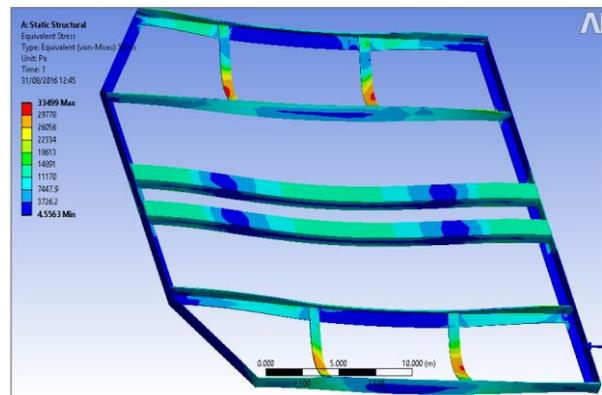
Pic 3: Von-Mises stress for steel chassis
