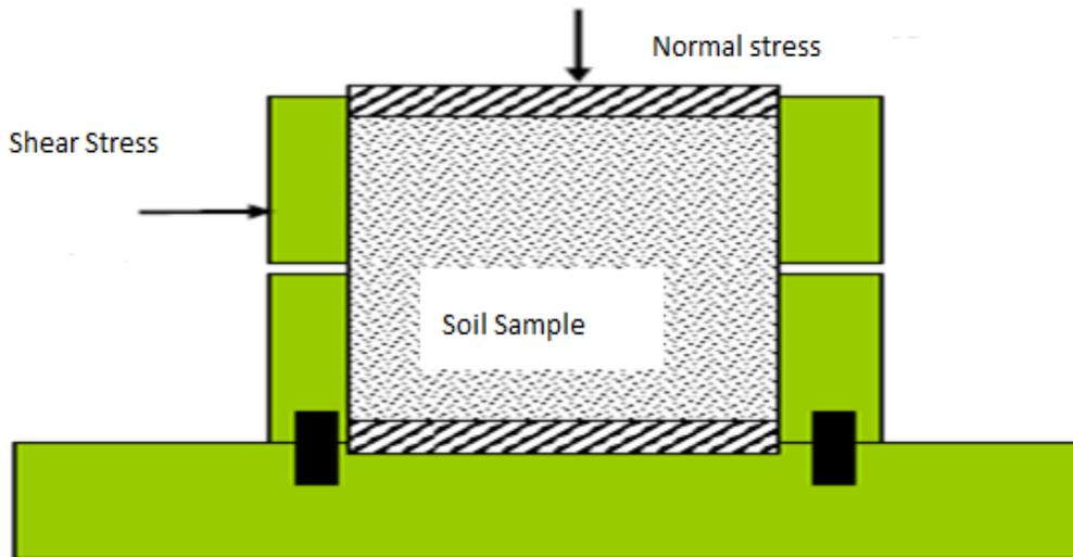
Figure 1: Test Apparatus
