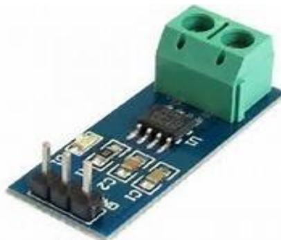
The device consists of a precise, low-offset, linear Hall sensor circuit with a copper conduction path located near the surface of the die. Applied current flowing through this copper conduction path generates a magnetic field which is sensed by the integrated Hall IC and converted into a proportional voltage.
