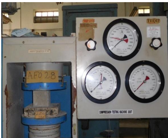
Fig.2 Testing of 100mm cube under compression
