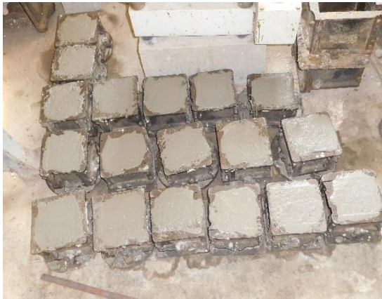
Fig.1 Cubes of 100mm under casting
