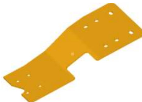
Fig.3. View of exhaust mounting bracket
