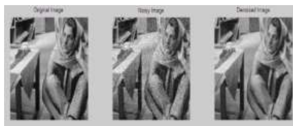
Fig 9 Barbara.jpg original, noisy and denoised image for \sigma=0.25 by wavelet transform
