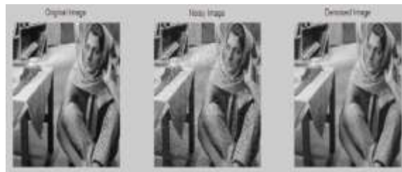
Fig 7 Barbara.jpg original, noisy and denoised image for \sigma=0.1 by wavelet transform
