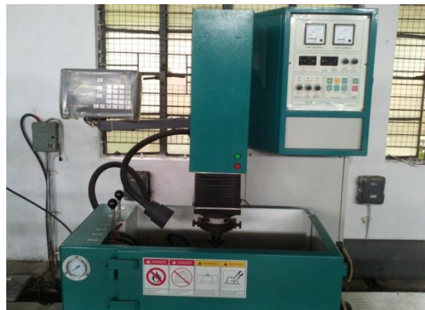
Figure 2: Electric Discharge Machine Setup
