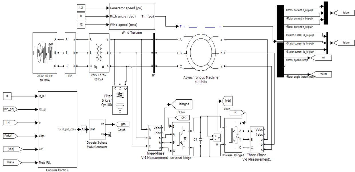
Figure 4 Simulation of diagram of DFIG system.
