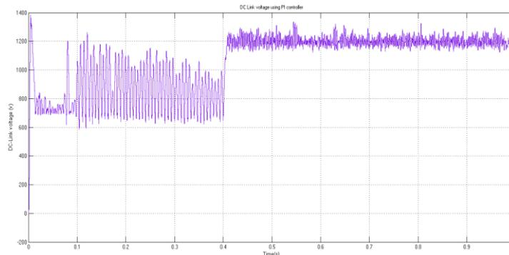
Figure 5 DC-Link voltages across capacitor using PI controller
