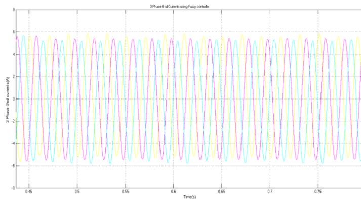
Figure 9- 3Phase Grid currents using Fuzzy logic controller
