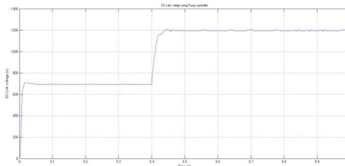
Figure 6- DC-Link voltage using Fuzzy controller
