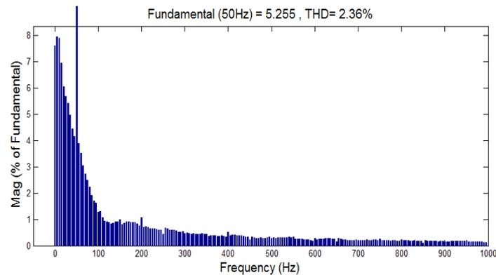
Figure 10 FFT Analysis of Grid currents using Fuzzy controller
