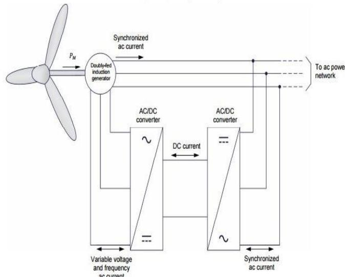
Figure 1 Block Diagram of DFIG
