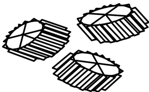
Figure (c) The bio-film carrier(K1)
