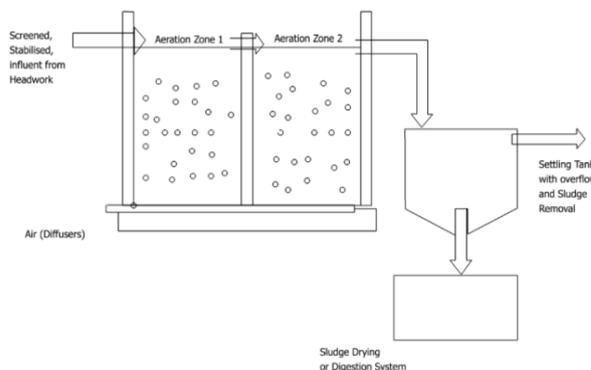
Figure 2 Moving Bed Biofilm Reactor process
