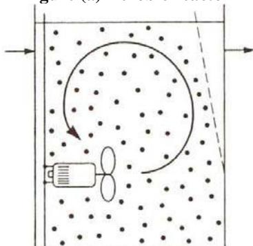
Figure (b) Anoxic and anaerobic reactor
