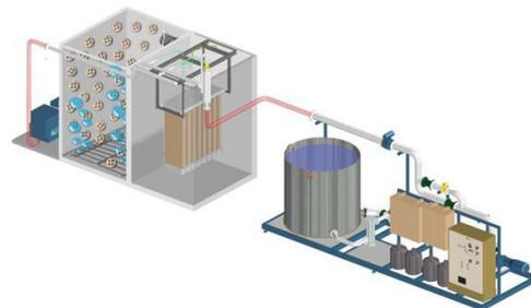
**Figure 1 shows the basic idea about the sewage treatment plant based on MBBR**
