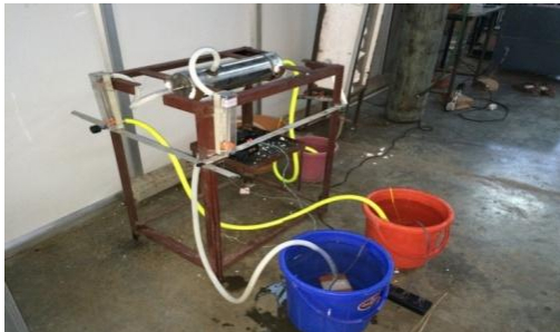
Fig 3.2. This is the original set up of equipment (for cold water in shell and hot water in tubes) on which experiment was conducted at J.D.I.E.T. Yavatmal.
