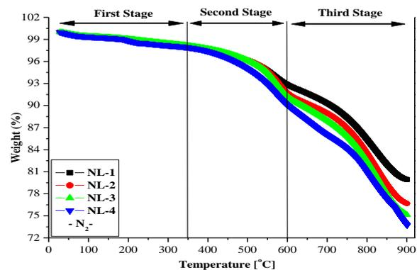
Fig. 1. TGA thermograms of friction composites materials
