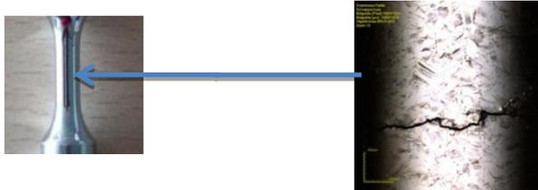
Figure 5. Cracks induced machine to stop experiment; specimen D10 at stress amplitude 230 MPa
