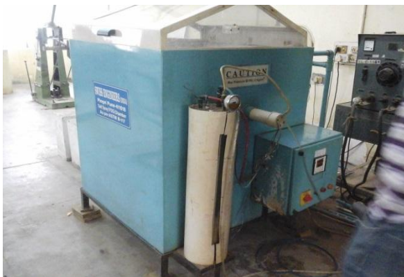
Fig. 3. Salt Spray Chamber ASTM B 117 (high pressure)
