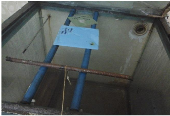
Fig. 6. Corroded Specimen in Salt Spray Chamber
