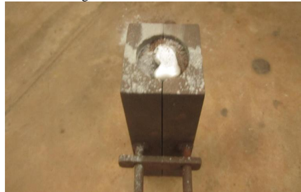
Figure 2. Composite casting in the cast iron die
