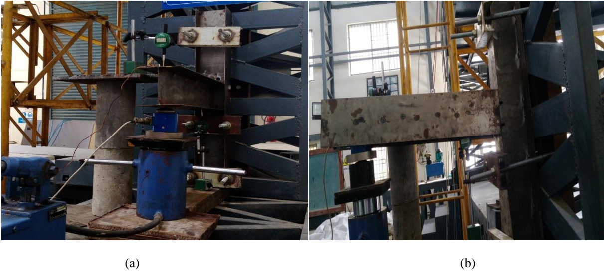
Fig 5 Experimental test setup Beam-Column specimens- I section (a) Web connection, (b) Flange connection.
