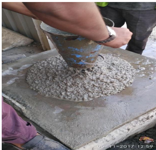
Fig.2. Flow Table Test
