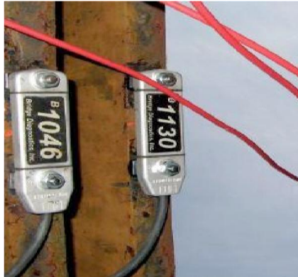
Figure 2: - Accelerometer and strain gauges used in Experiment
