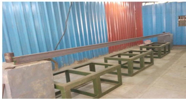
Figure 1: - ISLB 100 spanning 6m on which experiment is performed
