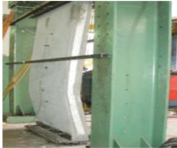
Fig. 11. Compression test result in bending at 700 KN
