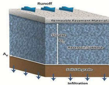
Fig. 2. Percolation Process of Permeable Concrete
