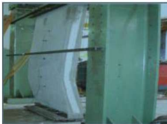
Fig. 12. Compression Test Result in Bending at 700 KN
