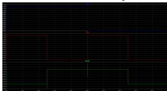
Fig 15: Waveform for XOR cell using Modified GDI cell
