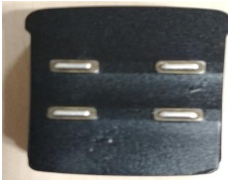
Fig. 1 4- channel Ag/AgCl electrodes used on the sensor
